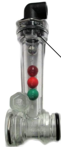
The low flow columns have a smaller interior diameter allowing a heavier ball to monitor a smaller flow.
