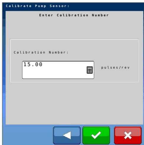
Check your pump's sensor pulses/rev calibration number. If you do not have one then disable the pump's sensor feature.
