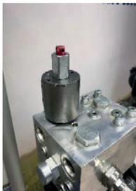
When the RED knob is pushed down, your pump system will be controlled by your controller.
