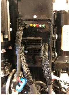
You should have a consistent **GREEN** light on signaling 12 volts. You should also have a blinking **BLUE** light signaling a PWM signal exists.
