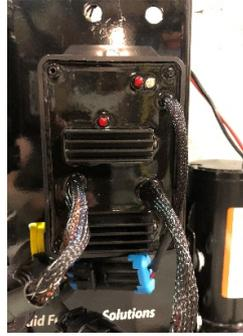
You Should have a blinking **RED** light signaling 12 volts (The light in the middle). This light should be solid **RED** when the system is running.
