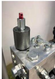
When the RED knob is up, your pump system is in manual mode.
