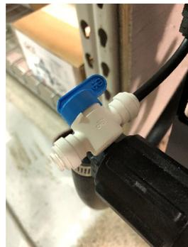
Opening the bleeder valve while the system is priming can let air escape your system that might be trapped. Keep this open until liquid starts to shoot out.
