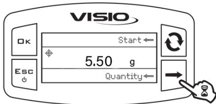
1) Press key for 2 seconds to open the manu for setting the filling quantity.
