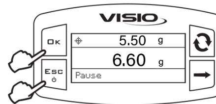
Tank filling can be interrupted at any time by pressing **ESC**. **Pause** message will be shown at the bottom of the display.
