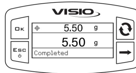
When set quantity is reached, filling stops automatically. **Completed** message will be shown at the bottom of the display.
