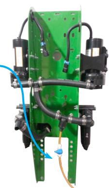
Pictured GX2 Dual Pump System – Blue prime valve is in the closed position
