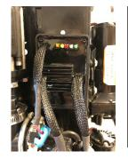
You should have a consistent GREEN light on signaling 12 volts. You should also have a blinking BLUE light signaling a PWM signal exists.
