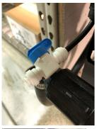
Opening the bleeder valve while the system is priming can let air escape your system that might be trapped. Keep this open until liquid starts to shoot out.
