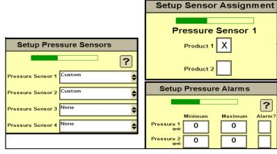
Sensors (such as pressure, pump RPM, spinner RPM) do not need to be assigned to a specific product if they are just being used to monitor a device and not to control it. AgXcel recommends that you NOT assign pressure and RPM sensors to a specific product. However, there may be times when you want to assign the sensor to a product.
